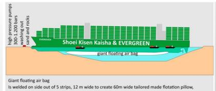
that is pulled under ship hall and pressurized by air form compressors.
